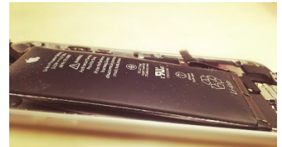
Figure 1: Swollen lithium-ion accumulator (source: SSHE)
